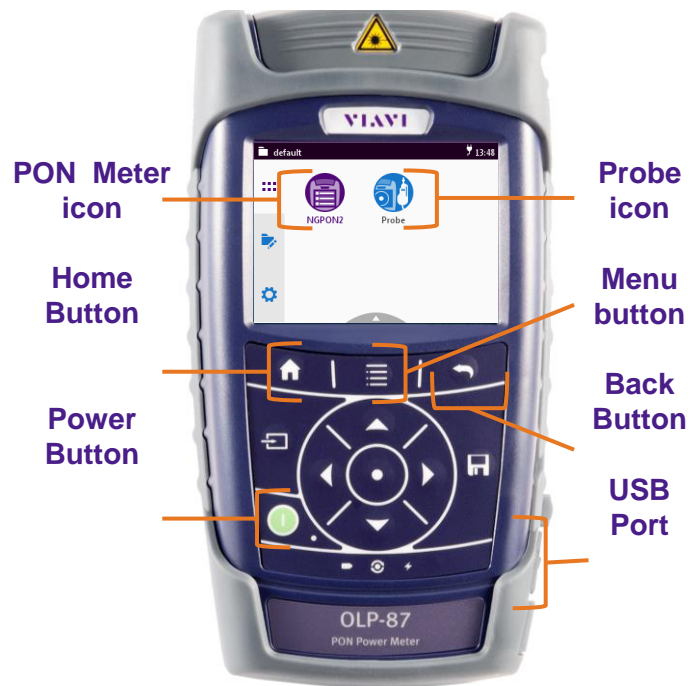
Figure 4: OLP-87, Front View
